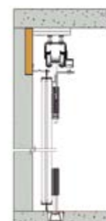
Posa soffitto in luce Installation in the opening Einbau in der Öffnung
