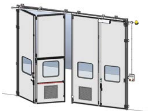
Sospeso senza guida a terra Hanging without floor track Freitragend, ohne Bodenführung
